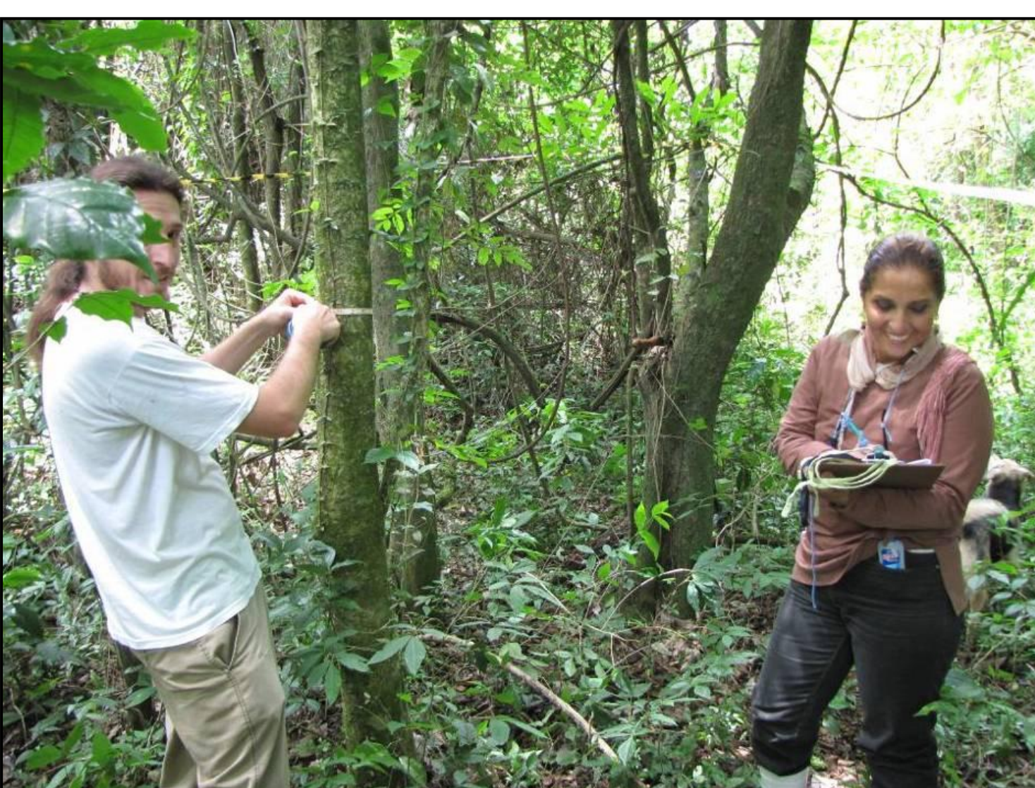
Figure 7: Measurement of the CAP (Circumference of tree measured at 1.30 m (at breast height) above the ground).
